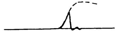
wave chopped by discharge on peak or on the front (to be interpreted by comparison with the characteristics of gas surge arrestors if any)
